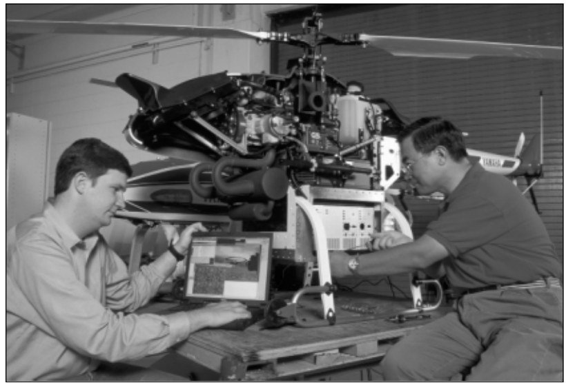
Aerospace Engineering’s Professor Eric Johnson (left) and Research Engineer Jeong Hur adjust components on GTMAX, Tech’s test bed unmanned aerial vehicle (UAV).
